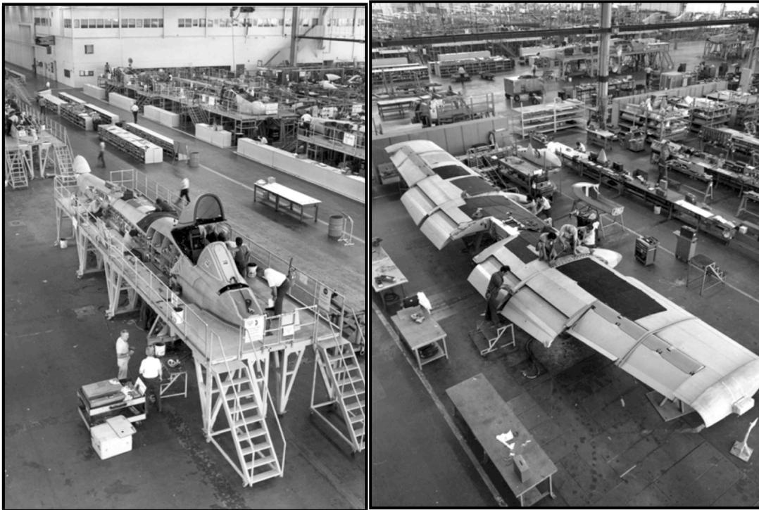
Figure 19. A-10 Fuselage and Wing Production<sup>10</sup>
