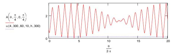
A proper calculation of the fraction of time that satellite is within range of target would integrate the function if  $(A(\theta) < \alpha, 1, 0)$  from  $\theta = 0$  to  $2\pi m$ , where m is the number of unique orbits:
